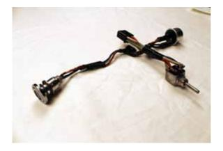
Modified hazard switch, indicator lamp, and flasher can assembly using terminals "C" and connector "B".
